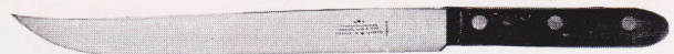
No. 1888 C.S.—9 inch Glazed Finish Carbon Steel Blade, Rosewood Handle, Nickel Silver Rivets, Scale Tang.
